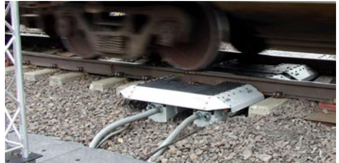
Wheel profile detectors capture critical information every time a train passes by.
